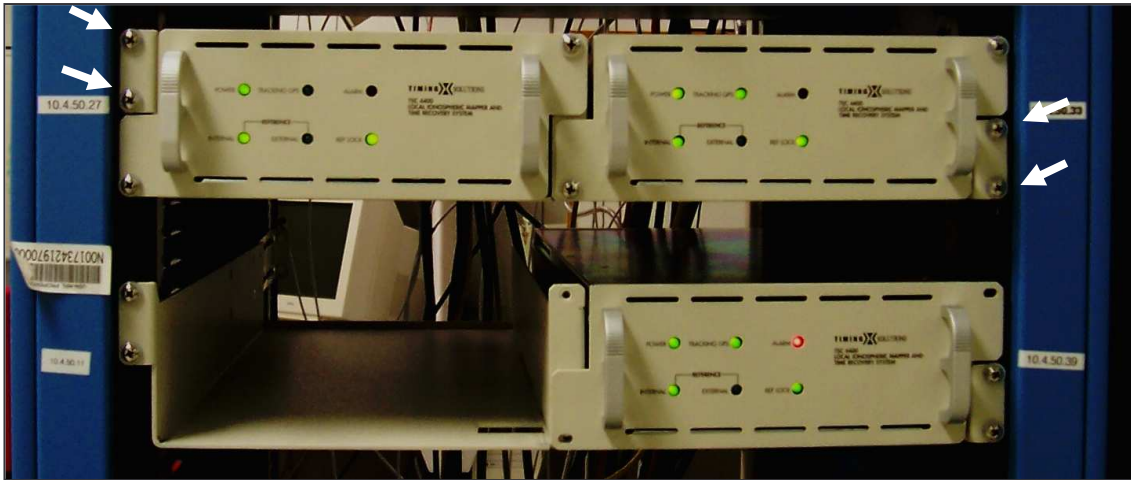
Figure 5-1. Two TSC 4400 units mounted side by side and a single TSC 4400 unit mounted on the shelf.
