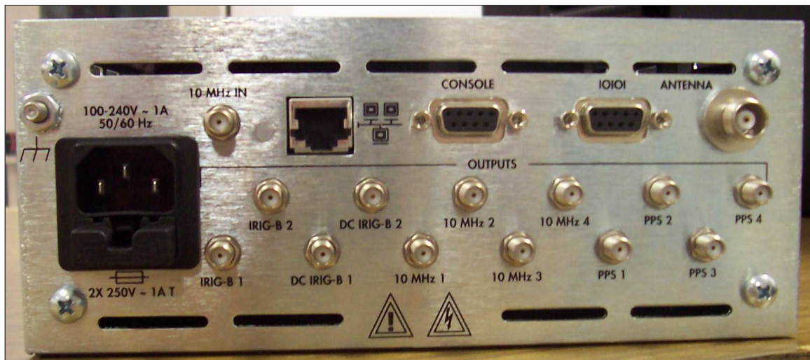
Figure 5-3. Rear panel of the TSC 4400.
